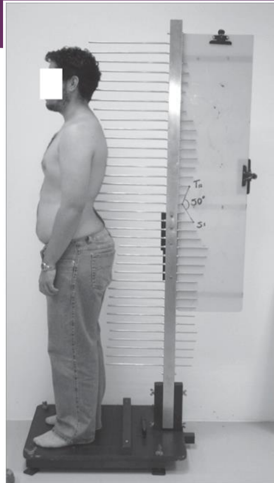
Figure 1. Kypholordometer - The subject's position and the demarcation of the most prominent points, regarding T12 and S1, and the least prominent points of the lumbar curvature.
